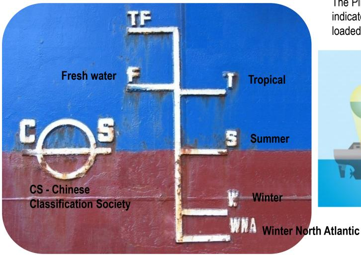
The Plimsoll Mark and Load Lines indicate how heavily a ship can be loaded.
