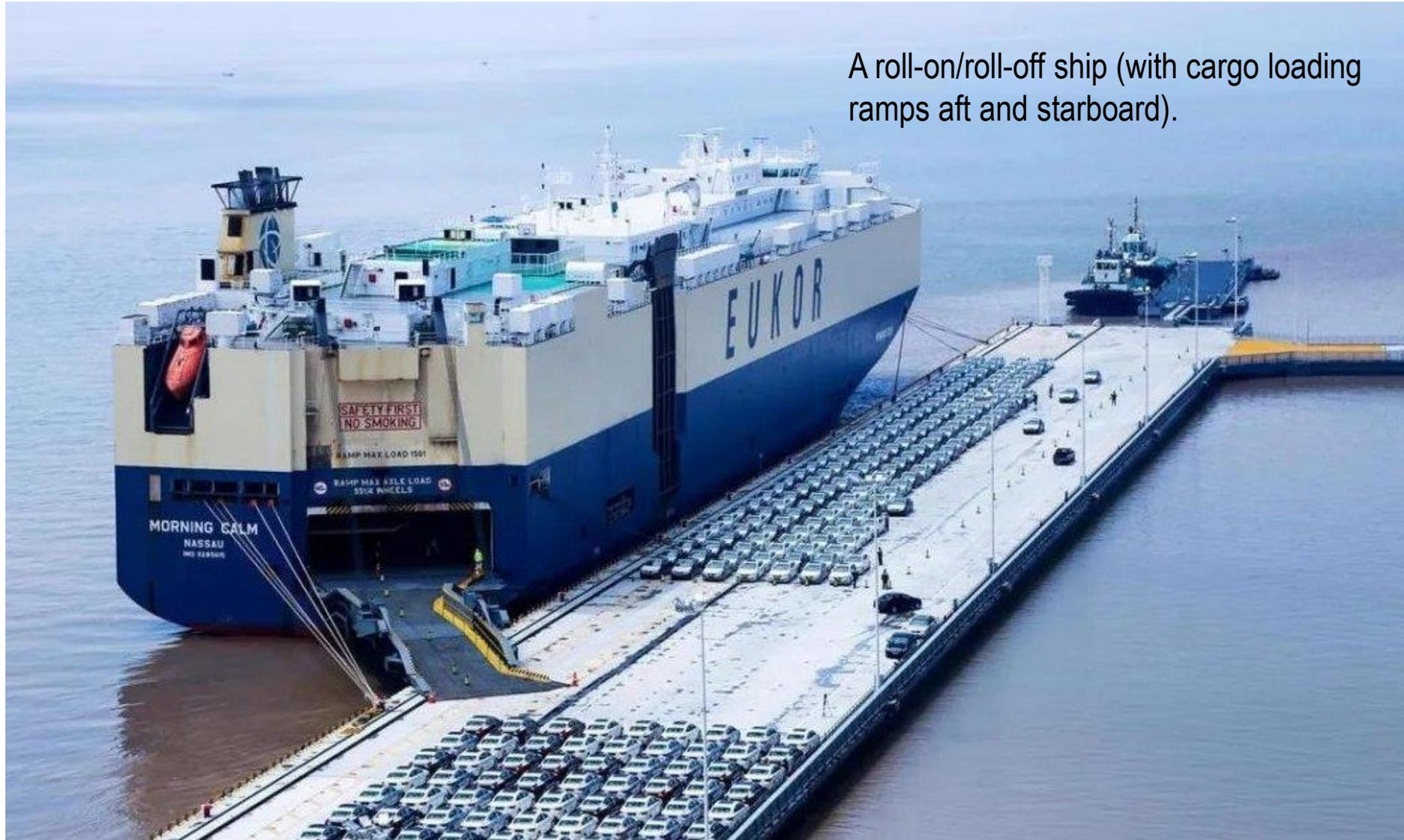
A roll-on/roll-off ship (with cargo loading ramps aft and starboard).
